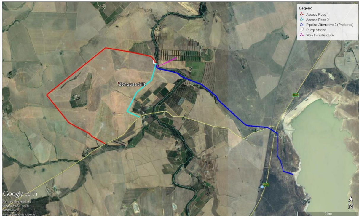
Figure 17: Proposed access to weir and pump station
